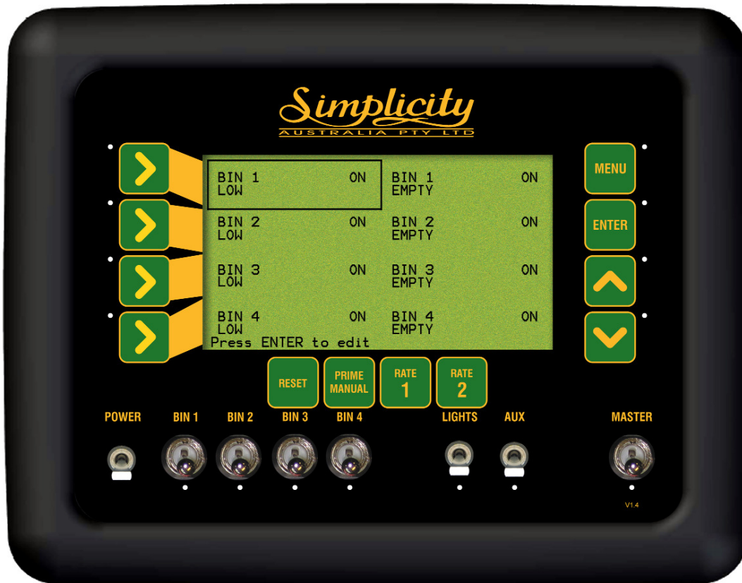
Bin Alarm Screen
